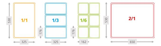
A 1/3 container is 325mm (same as 1/1) but just a third as wide (176mm), while a 1/6 is half the size again. 2/1 is twice the size of 1/1, measuring 530mm x 650mm.
