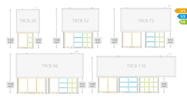
Note: even though drawer capacity of some TRCB units may appear to accept a larger than 1/1 GN pan, the drawer construction of these units are moulded specifically for this pan size as a way of strengthening the drawer and durability of the product.
