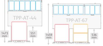
As standard, TPP products are supplied with 1 horizontal divider bar per drawer, facilitating 2x1/1 pans, 6x1/3 pans, or a combination of.
