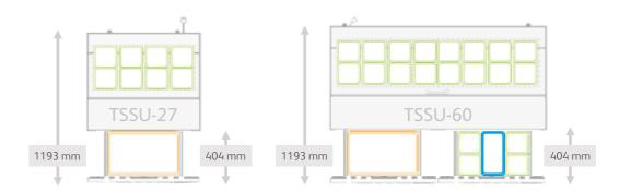
As standard, TSSU products are not supplied with any drawer divider bars. Drawers accommodate  $1x\frac{1}{1}$  or  $3x\frac{1}{3}$  pans without the need for additional bars.
