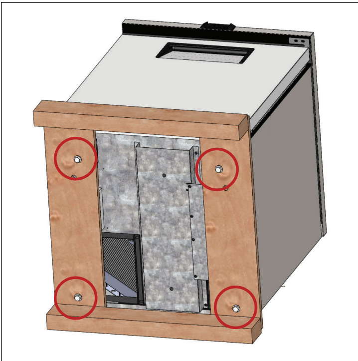
Fig. 3. Remove all shipping bolts.
